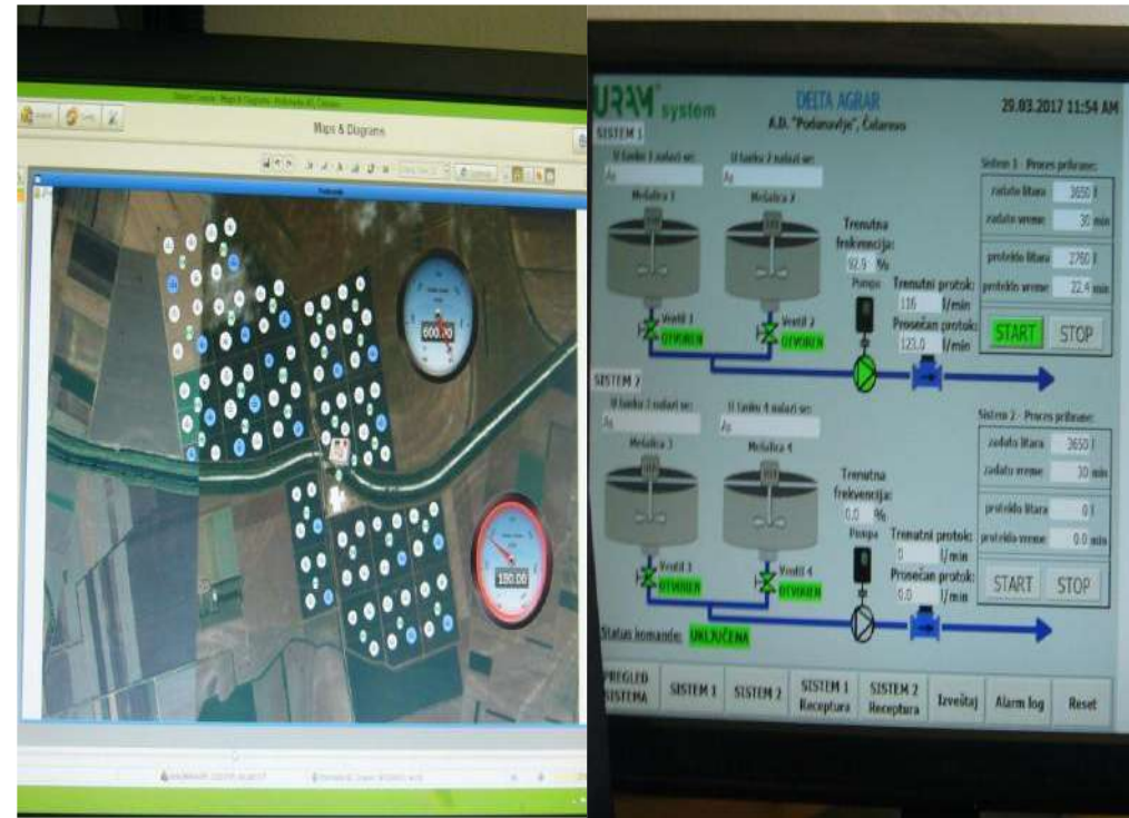
Figure 25. Smart irrigation and fertigation management in real time (Stričević, R., own archives)
